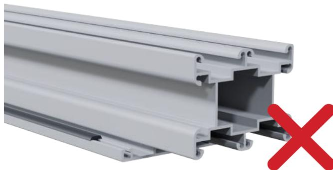
It should be noted that the seals used contract after installation in the profile channel. We recommend fitting the seals on both sides with an excess length of at least 25 mm and cutting them flush with the profile channel after the sealing have settled. In the case of seals with special lengths, we point this out in the installation instructions. Denominations are possible for the seals.
